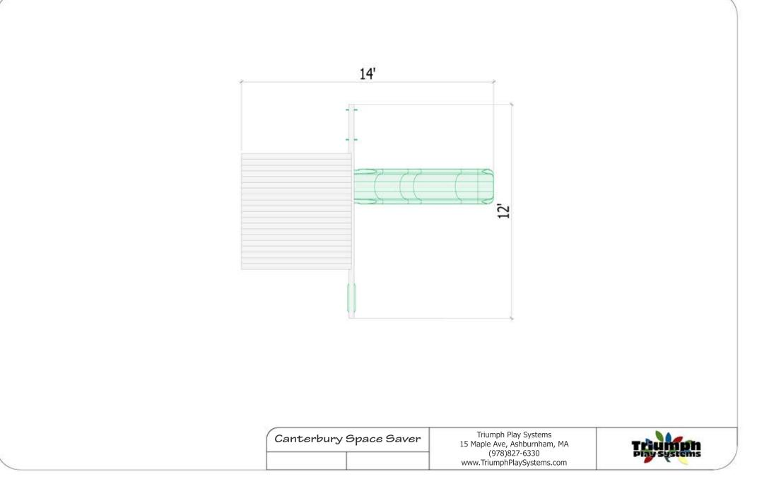
We recommend using a resilient play surface and allowing a 6-foot perimeter around the entire structure.
