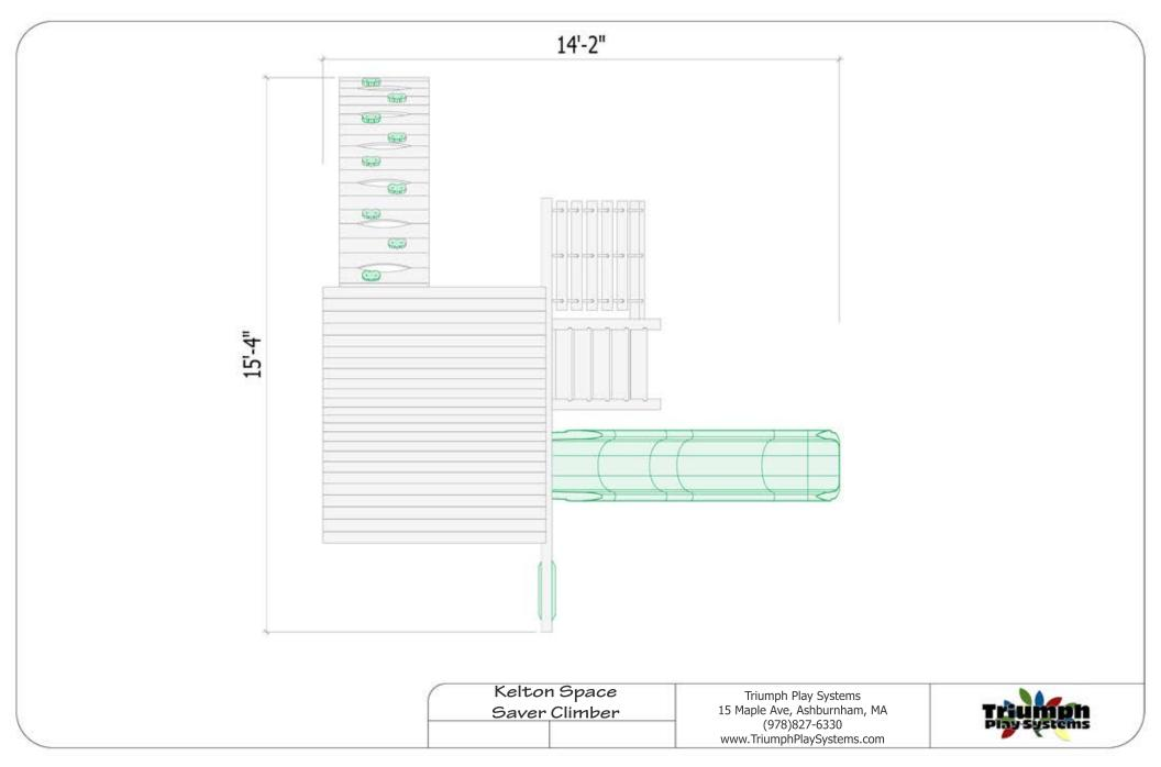
We recommend using a resilient play surface and allowing a 6-foot perimeter around the entire structure.
